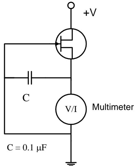
A 10% correction is included because  $I_d$  is slightly larger than zero.  $R_m$  is very small when the meter is on the current scale, hence  $V_{gs}$  is approximately zero, which means that
