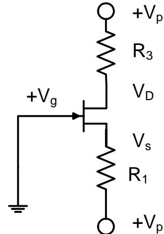
**6 - Observe  $V_s$  with a meter while you vary  $V_n$  from 0 to 25 volts. You will see that  $V_s$  changes as necessary so that the channel can conduct the current flowing through  $R_1$ . Give a brief explanation of how this self-adjustment occurs in your own words.**
