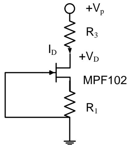
for  $R_1$  that is closest to the calculated value. Measure  $V_d$  and  $V_s$  and compare to that expected.
