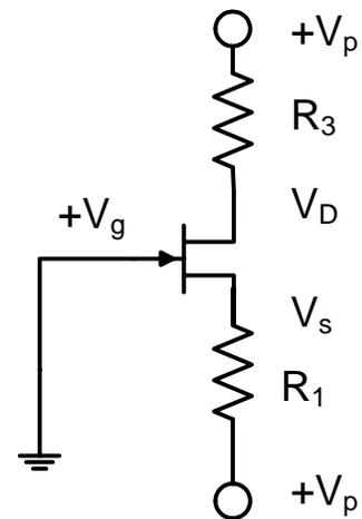
$V_T$  and  $I_{dss}$  given in the spec sheet. Use the  $I_d$  obtained with typical parameters in the first part of this problem as an estimate for the new  $I_d$  in eqn. (1.5), which in turn is used to estimate the new  $V_{gs}$ . This estimate is adequate because  $R_1$  prevents  $I_d$  from changing dramatically. Repeat for the minimum parameters given in the spec sheet. When  $V_n \gg V_{sg}$ ,  $I_d$  is relatively independent of the FET parameters because they only affect  $V_{sg}$ .
