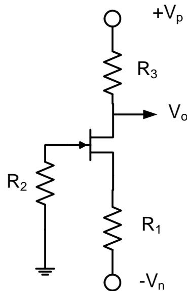
The maximum amplitude is obtained for a sine wave when the positive and negative limits are equal.  $I_d$  is then given by the following relation:
