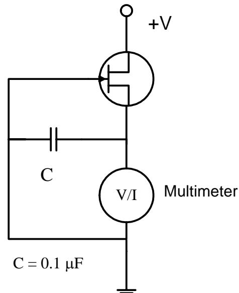
$$V_{meter} = V_{sg} = 0.9V_T \quad \text{Meter on voltage scale}$$
