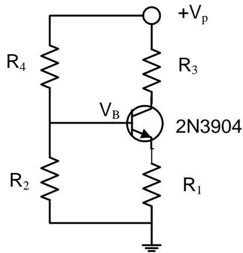
negligible, but the base current of a BJT can affect the divider. First we consider a case where the divider resistors are small, divider current large, so that  $I_b$  can be neglected. Next we increase the divider resistors to obtain a higher resistance at the input and include the effect of  $I_b$  on  $V_b$ .
